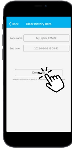
Select the zone, ensure the end time and click "Delete data". This will cause the app to clear the history of all the data until the selected end time
