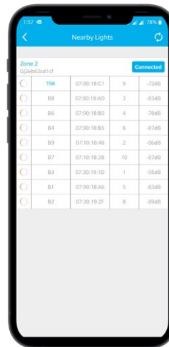
All the lights that are within the range can be seen along with important information which is helpful during commissioning.
