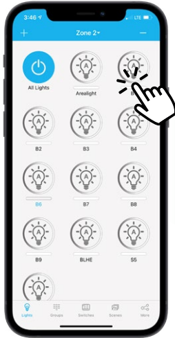
Long press the light icon to open up the individual light dimming settings.
