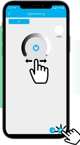
Adjust the dial to control the brightness. Tap the A at the bottom right to access Sensor settings
